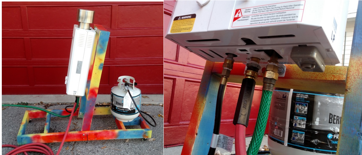
Figures A and B left to right. Figure A - Side view of the portable water heating system used for the intermediate testing. Figure B – Bottom view of the propane heater illustrating propane connection, incoming (green) and outgoing (red) water connections.
